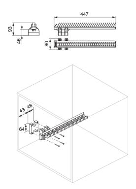
Montaje cinturonero Keeper Montaggio porta cinture Keeper Installation for Keeper belt rack
